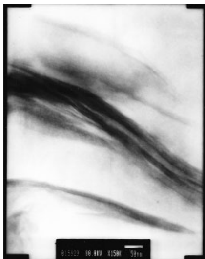
Figure 7 TEM micrograph of the cross section of PI-MMT.
